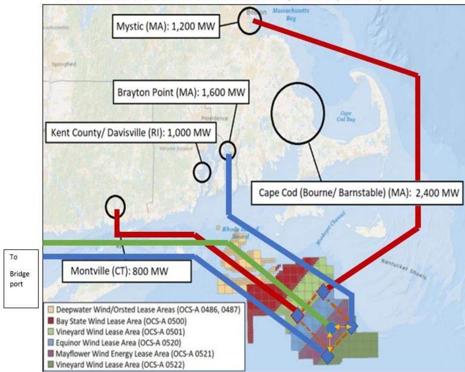
Dashed lines represent future potential interconnections between converters to increase offshore grid flexibility
